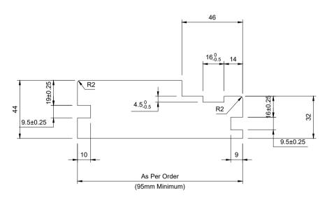
Extension Head Length = Lining Head Length Extension Head Rebate Length = Extension Head Length - 50mm Extension Head Rebate Depth = 9mm Extension Jamb Length = Lining Jamb Length + 15mm
